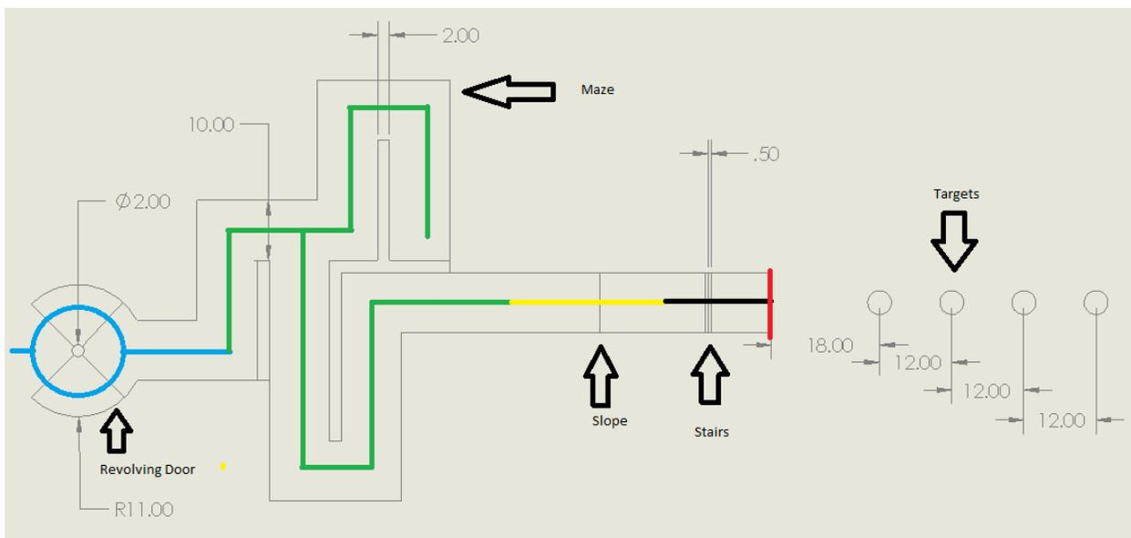
\*Course is drawn to scale. All measurements are in inches. The color used in the drawing will be the color of tape used in that area of the track. The walls are at least 3.5 inches tall.
